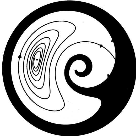
FIG. 3.1. Schematic representation of basin boundaries for attractors in the perturbed Poincaré map for the rotational motions of the parametrically excited mathematical pendulum. Shaded region is in the basin of attraction of the invariant torus.
