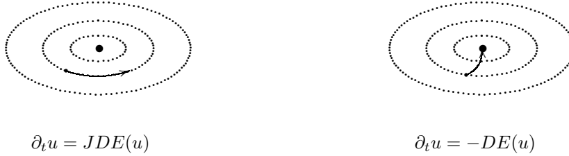
Fig. 2: Hamiltonian versus gradient systems (dotted lines are the level surfaces of the energy functional E ).
